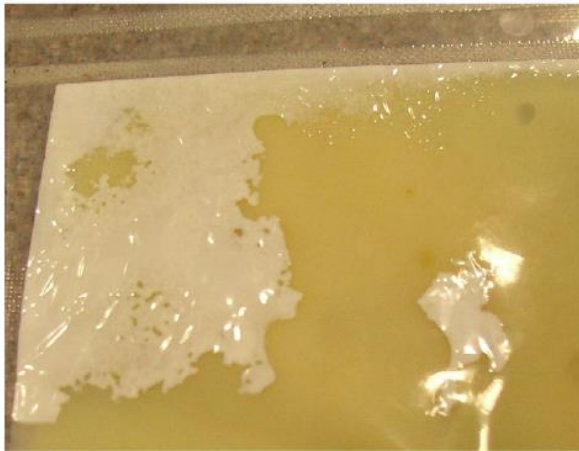
Fig. 2. Large delamination areas on PET-AlOx 12 µm/ON 15 µm/CPP 80 µm pouch after HPT processing.
